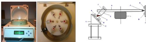
**Figure 1:** Prototype for bedside ABO determination including 2x3 assay units containing anti-A, anti-B and buffer as an internal control.
